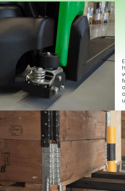
Easy long-side pallet handling. Twin fork wheels as standard, for reduced pressure on floors and easier and silent travel over uneven surfaces.
